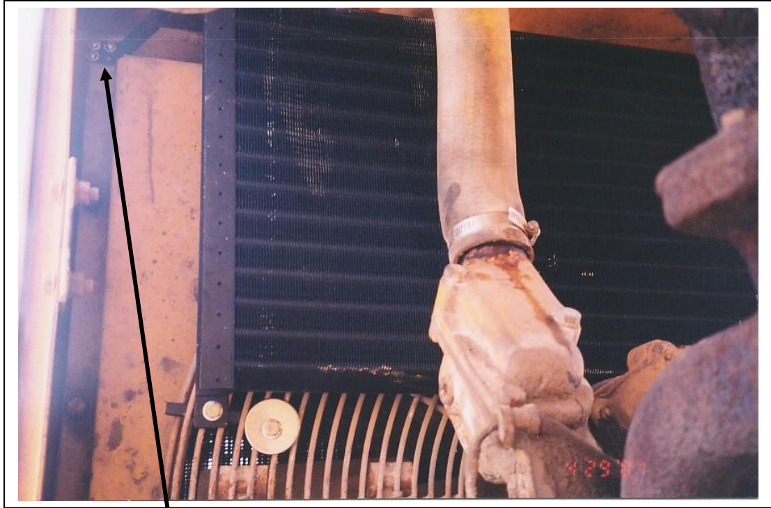
Upper condenser bracket screwed to radiator flange. (shown on 544E, similar for 624G)
